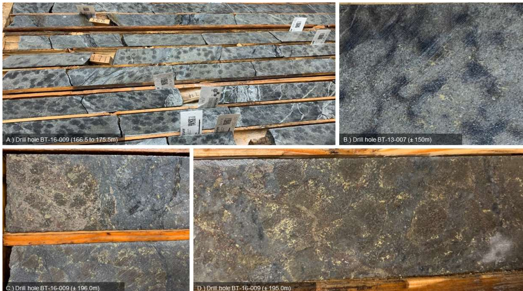
Figure 12.4 – Main Zone strongly altered ultramafic intrusion with gradual sulphide replacement (QP core review)
